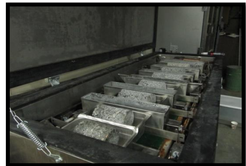
Figure 3: Testing Freeze-thaw Durability of Pervious Concrete
