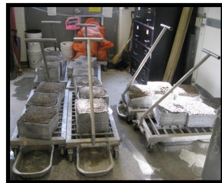
Figure 4: Pervious Concrete Slabs
