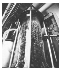
Glass Marble-filled Stripping Column
