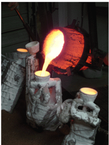
Fig. 5: The Lost-Wax Method
