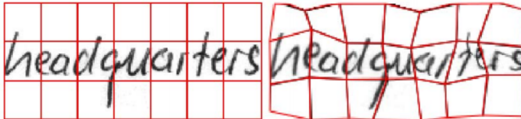
Figure 3.2 Word image with uniform grid, and perturbed grid with distorted image (Wigington 2017)
