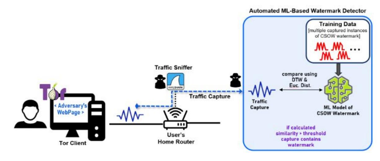
**LSTM Autoencoder** is trained on "normal" traffic (watermark) pattern only. Subsequently, the trained LSTM model is presented both normal and anomaly test data. This allows us to evaluate how well the model is able to both detect the **CSOW** in a randomly presented traffic instance, as well as to differentiate the learned **CSOW** profile from other webpages' traffic.
