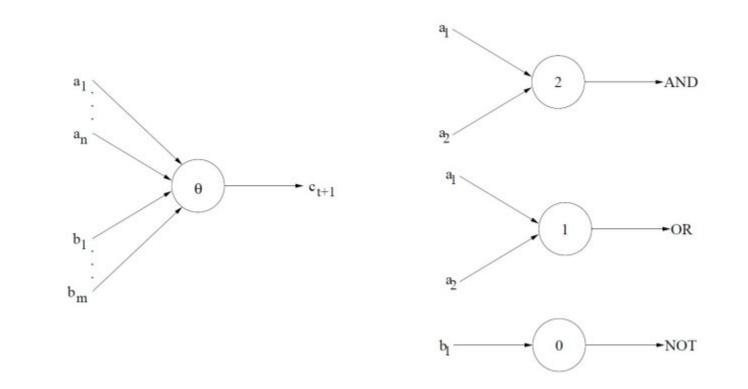
logic functions can be modeled by a network of MP-neurons
