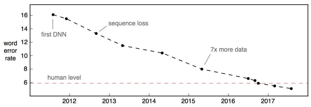
Improvements in word error rate over time on the Switchboard conversational speech recognition benchmark. The test set was collected in 2000. It consists of 40 phone conversations between two random native English speakers.
