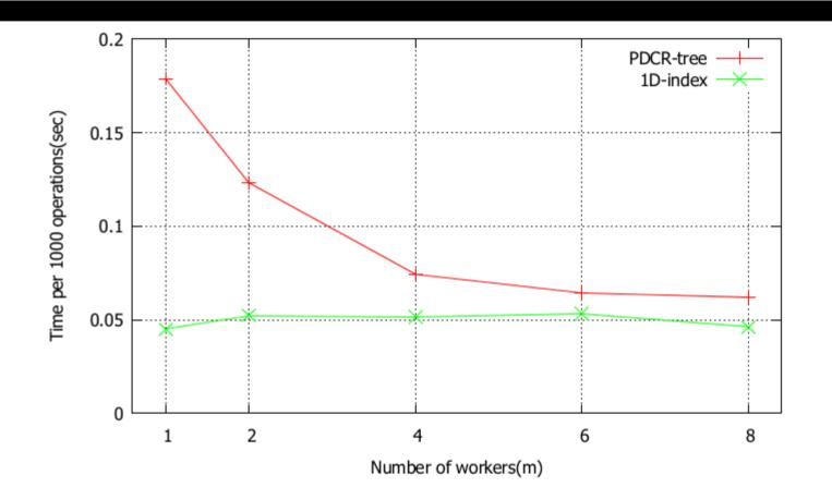
Time for 1000 insertions as a function of the number of workers. (N = 40Mil, d = 8,  $1 \le m \le 8$ ) N: database size, d: # dimensions, m: # workers
