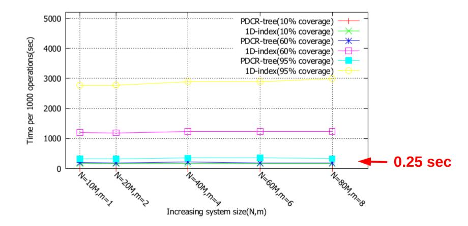
Time for 1000 queries as a function of system size: N & m combined.  $(10Mil \le N \le 80Mil, d = 8, 1 \le m \le 8)$
