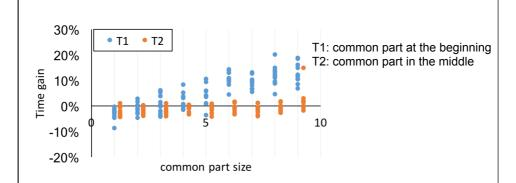
200 sets of workflows automatically generated of the following configuration: One common part of 1–10 nodes; Number of workflows in a set - 2–5; Workflow size - 20-50 vertices; Common part operators [blocking, nonblocking, restrictive] - [25-75%, 25-75%, 25-75%].
