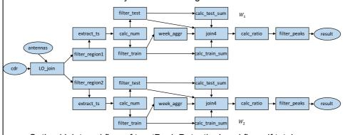
Optimal joint workflow of two 'Peak Detection' workflows if total selectivity of filter\_region1 and filter\_region2 is high
