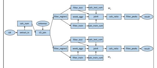
Optimal joint workflow of two 'Peak Detection' workflows if total selectivity of filter\_region1 and filter\_region2 is low
