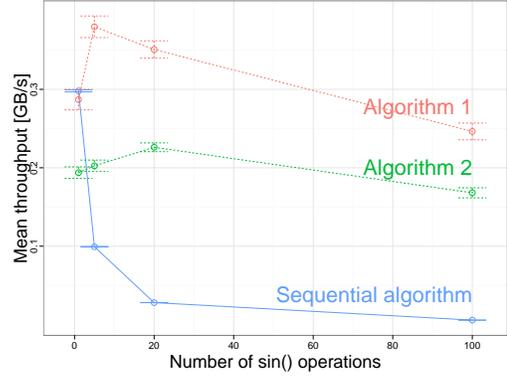
Figure 6. Throughput analysis - effect of computational load.
