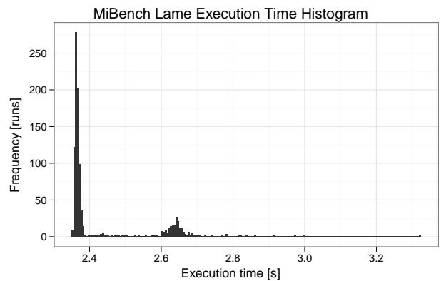
Figure 7: Density plot of the execution time of the MiBench lame program.
