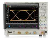
**Problems it solves:** I to look at fast signals in the time domain, analyze jitter, or understand timing relationships in picoseconds.
