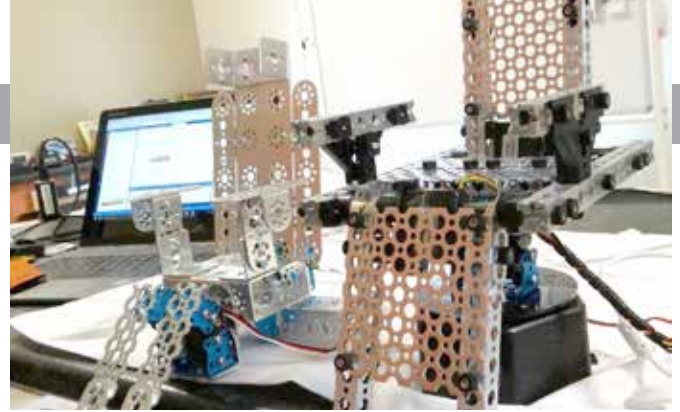
Above: The latest version of RoboChair is made of TETRIX® PRIME parts and servos, with the exception of the base. Below: Livingstone decided to paint his RoboChair model red to give it a warm, comforting look and feel.
