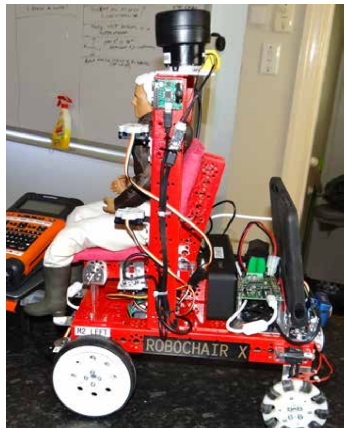
Above: The latest version of RoboChair is made of TETRIX® PRIME parts and servos, with the exception of the base. Below: Livingstone decided to paint his RoboChair model red to give it a warm, comforting look and feel.
