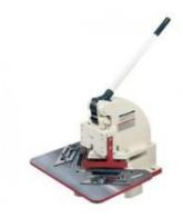
This piece of equipment is a hand operated corner notcher used in the fabrication of pans and boxes. It cuts 90 degree notches to facilitate bending flat sheets into a box or pan.
