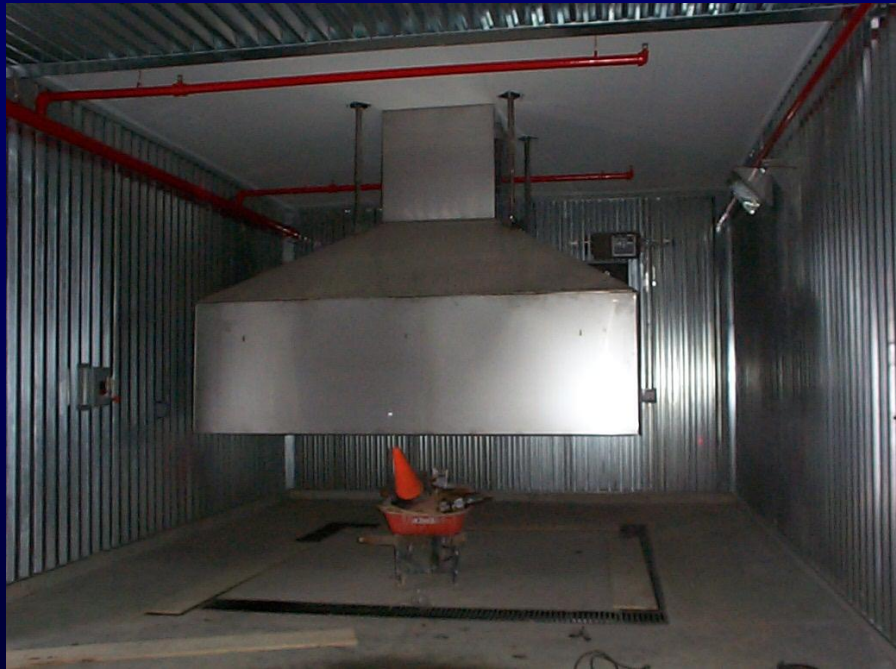
Large Cone Calorimeter 2MW fire test area
