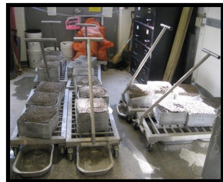
Figure 4: Pervious Concrete Slabs
