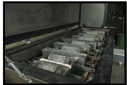
Figure 3: Testing Freeze-thaw Durability of Pervious Concrete
