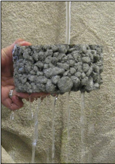
Figure 1: Pervious Concrete Pavement
