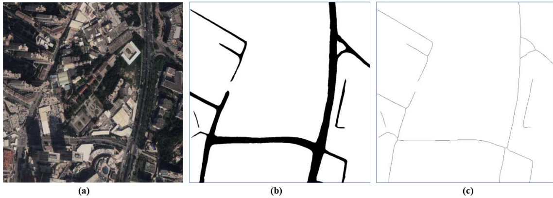
Fig. 14. Road centerline extraction from Google Map imagery. (a) High-resolution Google Map image captured in Xiamen, China. (b) Road extraction results using the D-LinkNet model. (c) Road centerline extraction results using the morphological thinning algorithm.
