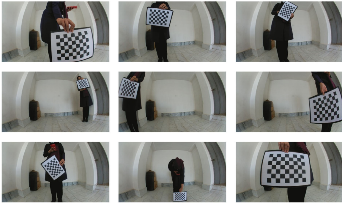
FIGURE 3 Example of images used to calibrate the fisheye image. [Color figure can be viewed at wileyonlinelibrary.com ]
