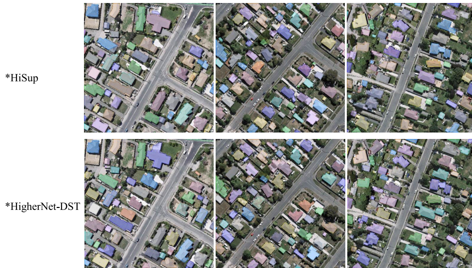
Fig. 7. Rooftop delineation results on the WHU Building Dataset obtained using the *HiSup and *HigherNet-DST.
