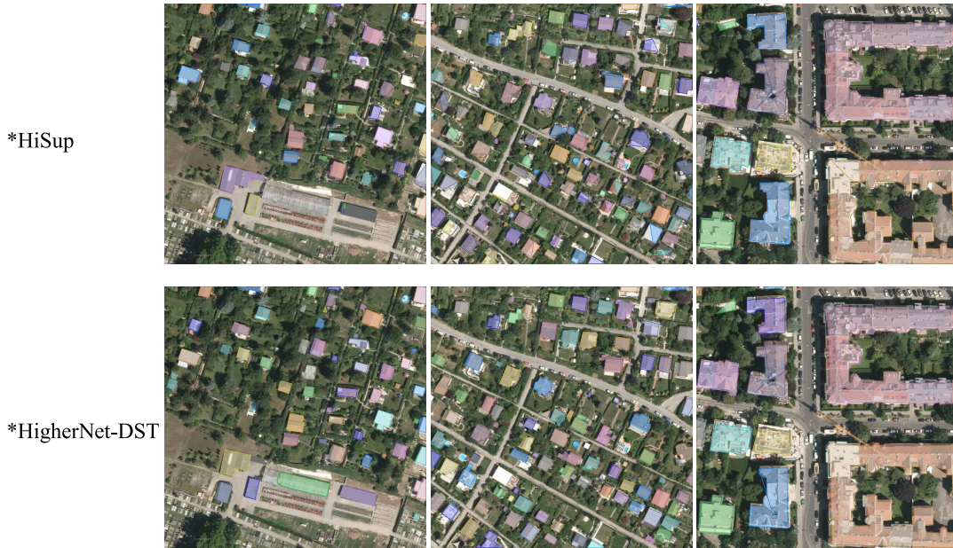
Fig. 6. Rooftop delineation results on the Inria Building Dataset obtained using the *HiSup and *HigherNet-DST.
