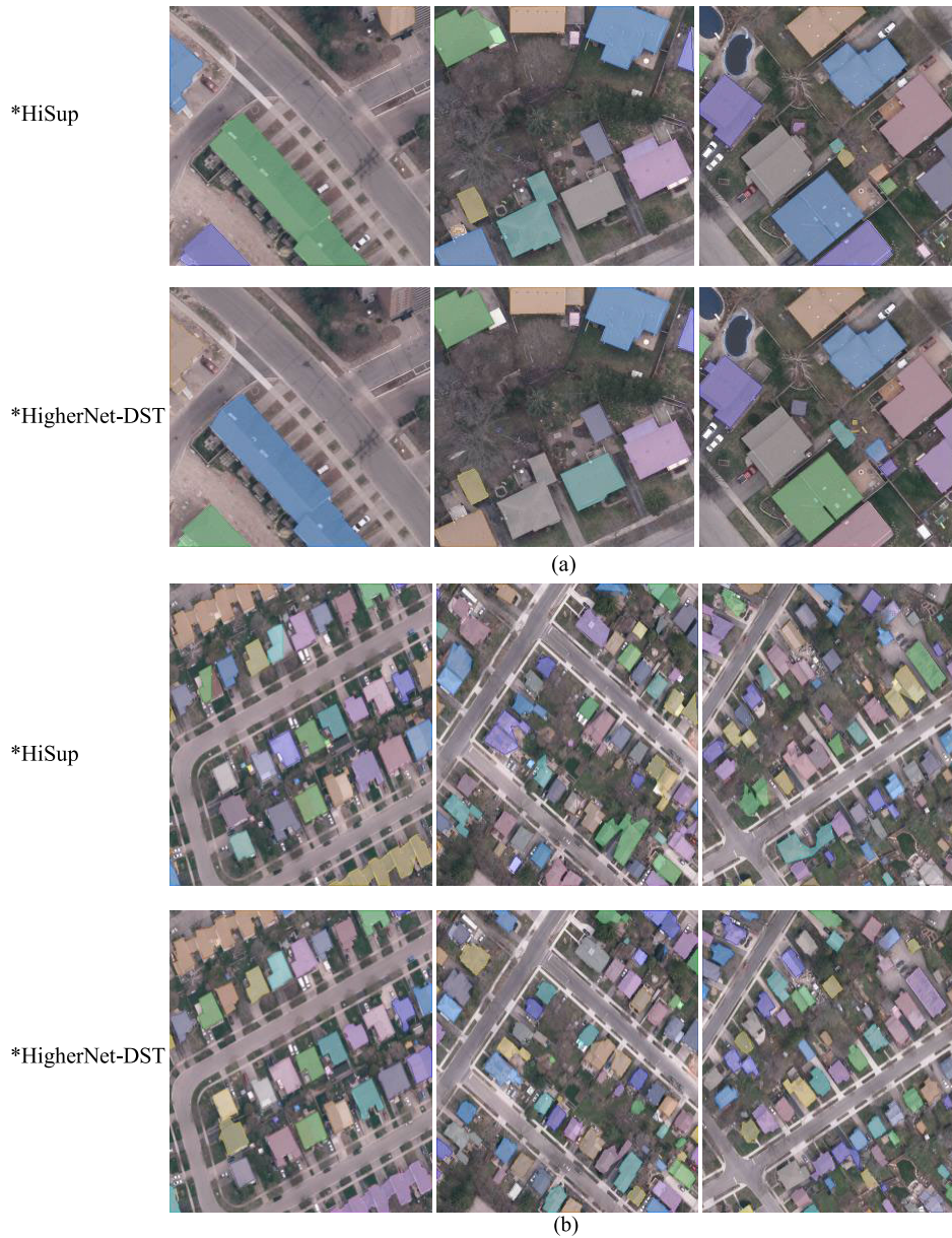
Fig. 8. Rooftop delineation results on the WBD obtained using the *HiSup and *HigherNet-DST. (a) Rooftop delineation results on the 0.12 m/pixel WBD. (b) Rooftop delineation results on the 0.30 m/pixel WBD.
