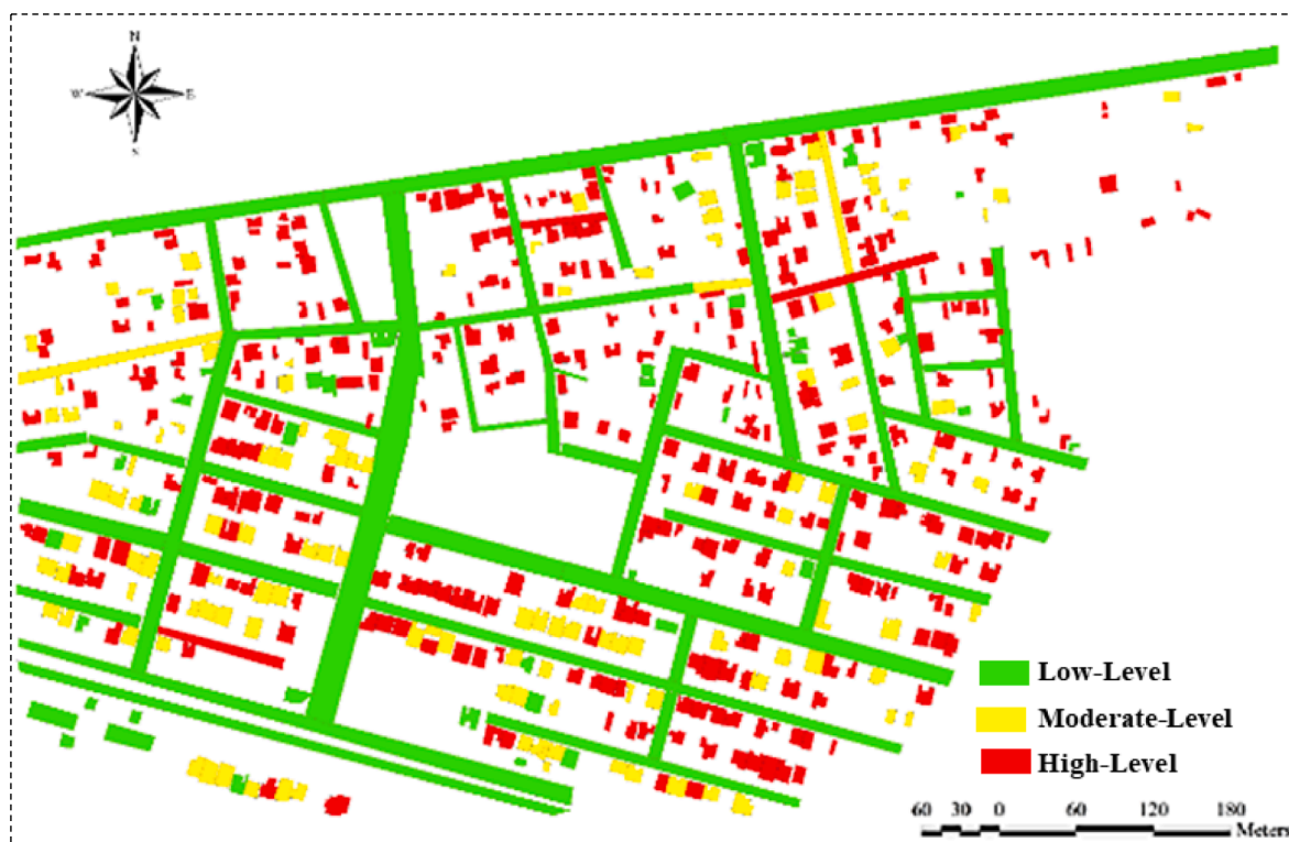
Fig. 13. Final damage map of the test area for the Bam dataset using the proposed BR-DMG process with the three levels of damages.
