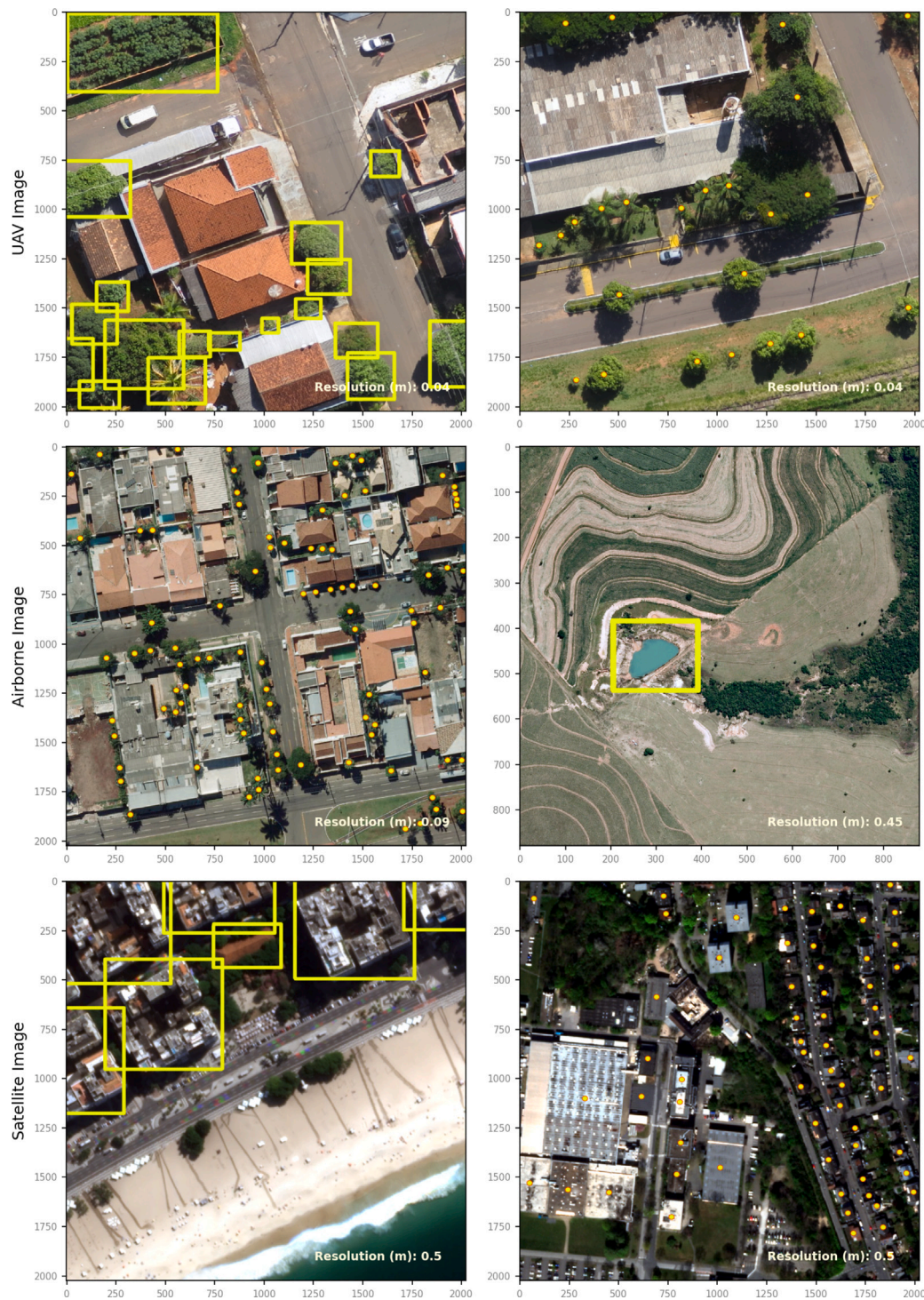
Fig. 2. Collection of image samples utilized in our research. The top row features UAV-based imagery with bounding boxes and point labels, serving as prompts for SAM. The middle row displays airborne-captured data representing larger regions, with both points and a rectangular box provided as model inputs. The bottom row reveals satellite imagery, again with bounding boxes and points as prompt inputs, offering a trade-off between lower spatial resolution and wider area coverage.
