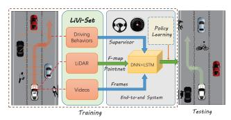
Figure 1. LiDAR-Video Driving dataset: a benchmark for polices learning in autonomous driving.
