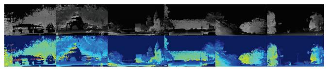
Figure 6. Examples of gray and jet feature maps. First row of this figure is gray feature maps and second row is the corresponding colored feature maps using jet color map. Depth information and spatial information (pedestrians, vehicles, trees, traffic lights, bridges, buildings and so on) can be obtained implicitly from maps.
