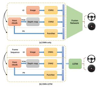
Figure 8. Network architecture of our prediction models.
