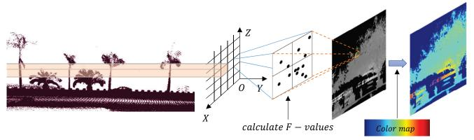
Figure 7. The pipeline of extracting feature maps from raw point clouds. Firstly, split XOZ plain into small grids, one of which is corresponding to specific one pixel in feature maps. Secondly, group raw points by projecting points into grids in XOZ. Then calculate feature values (F-values in figure) in each grid. Finally, generate feature maps by visualizing feature matrix and rendering with jet color map.
