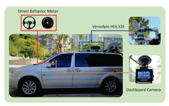
Figure 2. Our data collection platform with multiple sensors.
