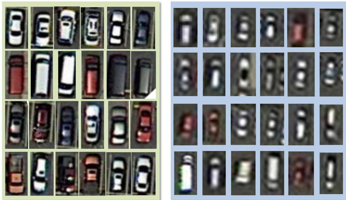
Fig. 6. Examples of vehicles extracted from low (left) and high (right) resolution imageries.
