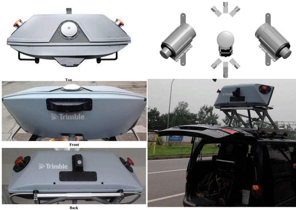
Figure 2. A system configuration of a Trimble MX-8. The system includes two Riegl® VQ-250 laser scanners, four Point Gray Grasshopper® GRAS-5055C CCD cameras, and a set of navigation system containing two GNSS antennas, an IMU, and a DMI. (Guan et al. 2013).
