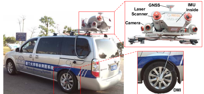
Fig. 4. Illustration of REIGL VMX-450 mobile LiDAR system and its configurations.
