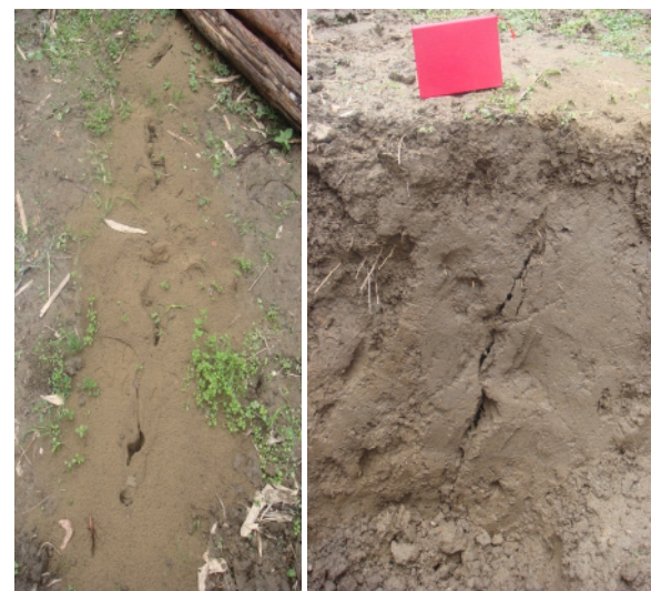
Figure 7 Sandblast body alignment from ground fissure caused by earthquake (left photo). Trench for research of southern segment of LFZ (right photo).
