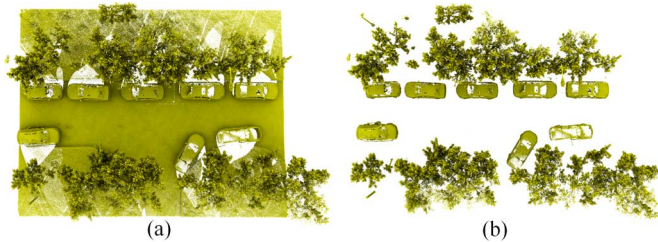
Fig. 8. (a) Raw point cloud. (b) Off-ground points after ground removal.
