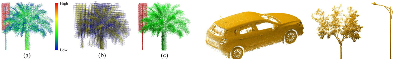
Fig. 7. (a) Cluster containing two overlapped objects rendered with intensity information. (b) Voxelization of the cluster by using the octree partition strategy. (c) Bipartition result of the cluster.
