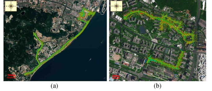
Fig. 10. Surveyed areas and the collected point cloud data sets. (a) Ring Road South data set. (b) Software Park Phase II data set.
