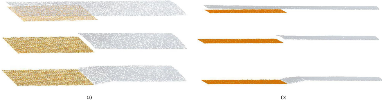
Fig. 11. Smoothing fusion based on progressive migration at two views as well as (a) and (b). The three rows in (a) and (b) represent the aligning, blending, and smoothing results of cross-source validated point clouds. 3D data of the orange yellow color represents TLS point cloud, the gray color represents SFM point cloud.
