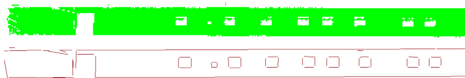
Fig. 13. Line extraction results on wall point cloud.
