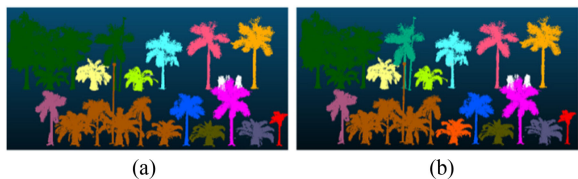
Fig. 9. Segmentation results of the region growing using (a) number of neighbor = 20, and (b) number of neighbor = 10.
