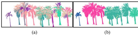
Fig. 8. Results of the Euclidean distance clustering. (a) 0.1-m distance threshold. (b) 0.3-m distance threshold.
