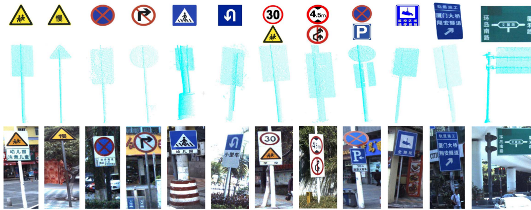
Fig. 9. Illustrations of parts of traffic sign point clouds and related images in our landmark dataset.
