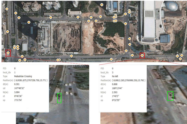
Fig. 11. Traffic sign landmarks with semantic and spatial properties visualized over an orthophoto in GIS.
