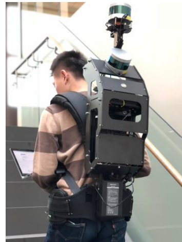
Fig. 3 Scanning an indoor using a backpack LiDAR.
