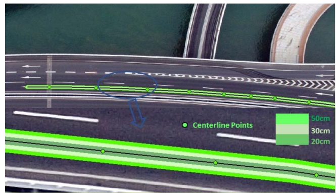
Fig. 17. Lane centerline validation results using user-defined buffer zones.
