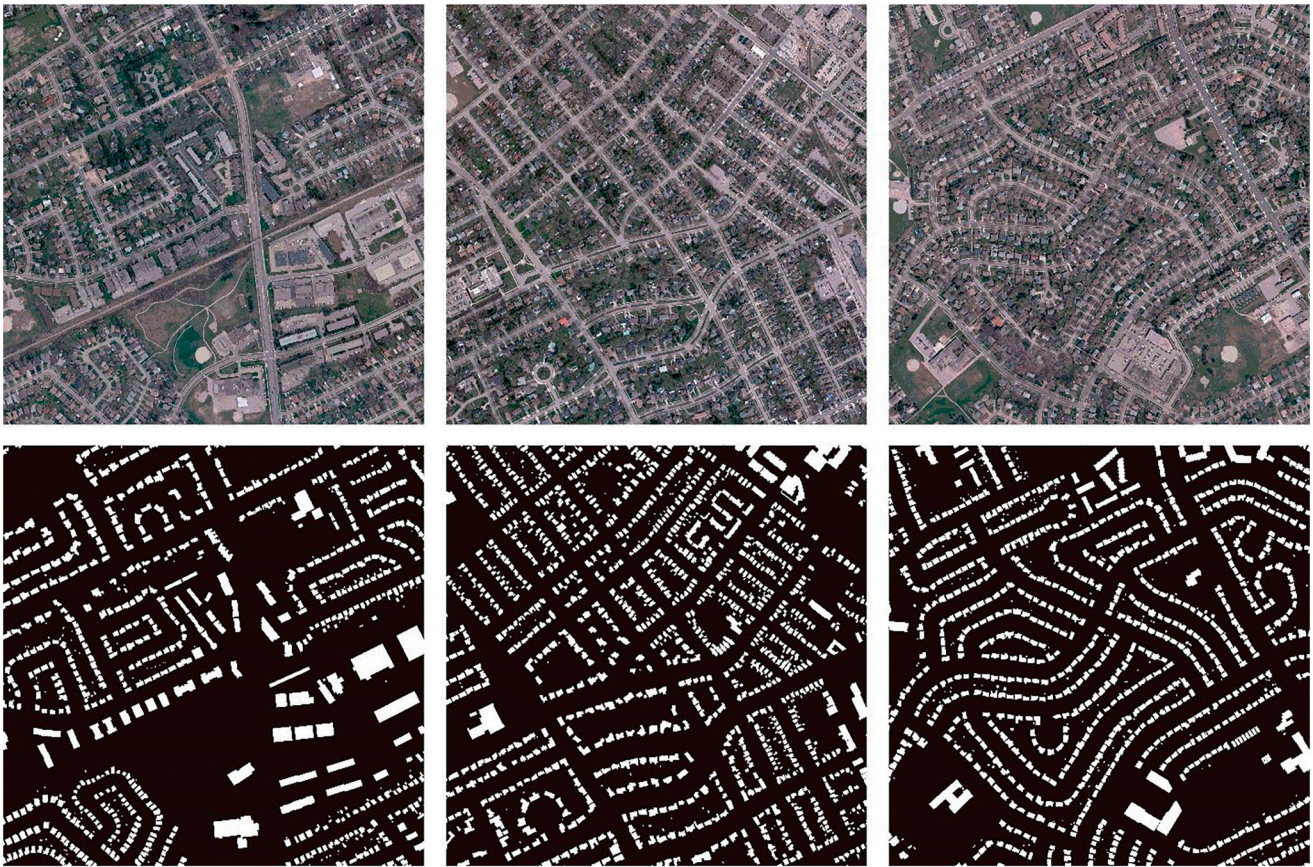
Figure 8. RGB color aerial orthoimages (top row) and their corresponding reference data (bottom row: labeled building rooftops).
