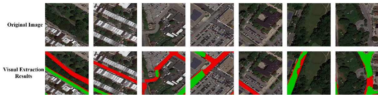
Fig. 11. Several wrong extraction examples of our method on LRSNY dataset. Green represents the right extraction and Red represents the wrong extraction. (For interpretation of the references to color in this figure legend, the reader is referred to the web version of this article.)
