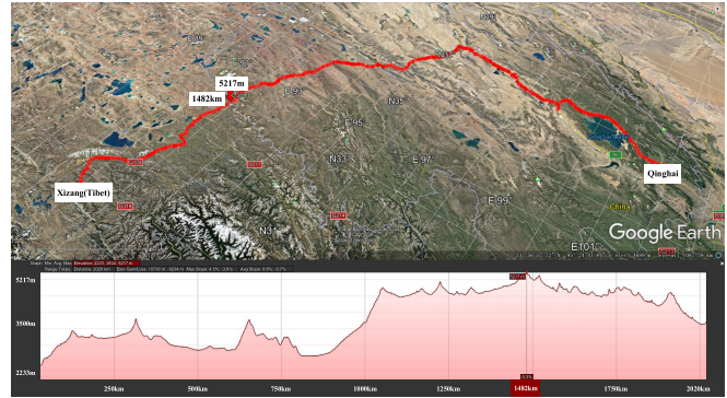
Fig. 4. The detail information of the Qinghai-Tibet Highway in Google Earth. The red line in the map represents the main road of the Qinghai-Tibet Highway, and the line chart below the map illustrates the elevation variance.
