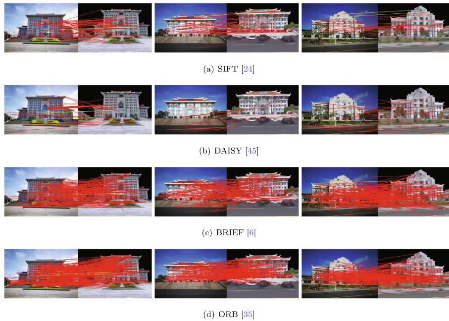
Fig. 3. The failed matching results between ground camera images and rendered images by using SIFT [24], DAISY [45], BRIEF [6] and ORB [35]. Each pairs is the corresponding cross-domain images, the left is ground camera image, the right is rendered image. The yellow lines represent the right match and the red lines represent the wrong match.
