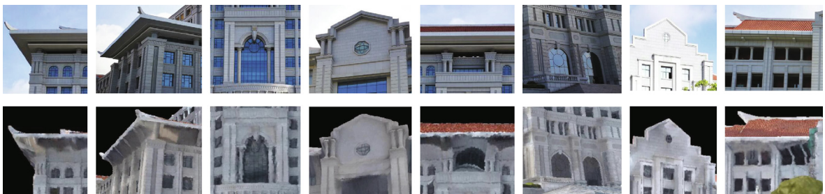
Fig. 10. Matching cross-domain image patch pairs. Top: ground camera image patches. Bottom: rendered image patches.
