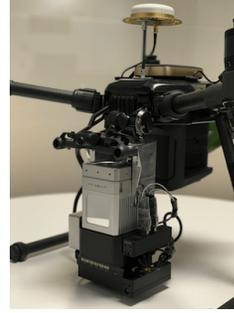
**Fig. 2.** UAV LiDAR system with Livox Mid-40<sup>1</sup>
