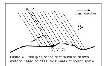
pushbroom cameras such as the ADS40 and STARIMAGER are all calibrated with focal plane coordinates of each CCD detector respectively provided. Therefore, the CPPS definition actually does not exist under this condition, or by definition, the CPPS is not ideally "plane" but irregular "surface" instead, which in fact results in rather complicated work for the rigorous parametric presentation of CPPS.
