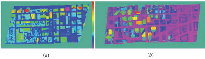
Figure 4. Test data I: point-clouds (a) and (b) from 'Downtown Toronto' data set.
