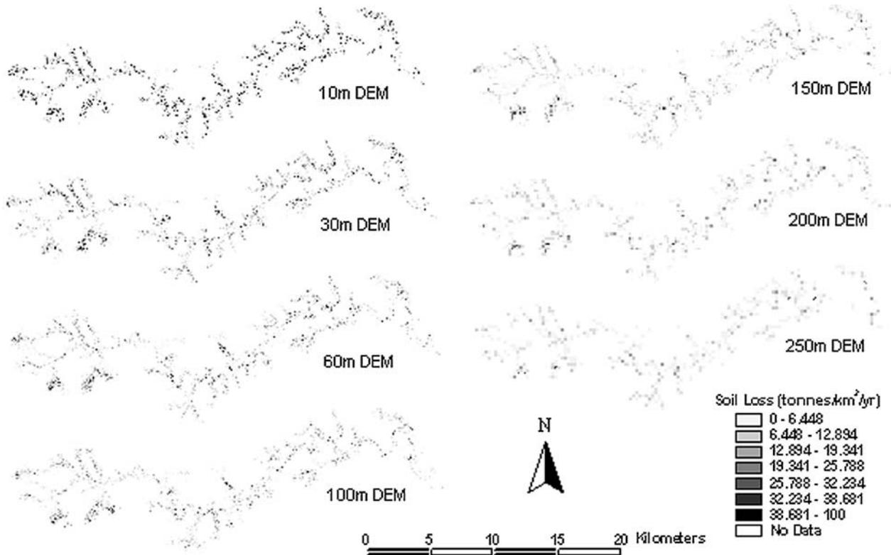
Figure 7. Distributions of cell contribution to total soil loss at different DEM resolutions.
