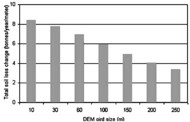
Figure 9. Sensitivity of total soil loss estimation to DEM grid size.
