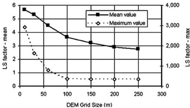
Figure 4. The *LS* factor versus DEM grid size.
