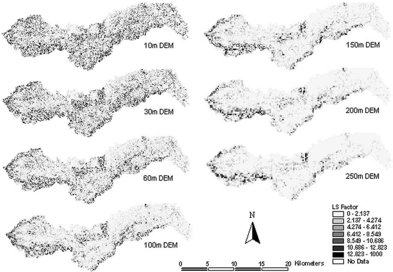
Figure 3. Distributions of the *LS* factor value for the DEMs of different resolutions.
