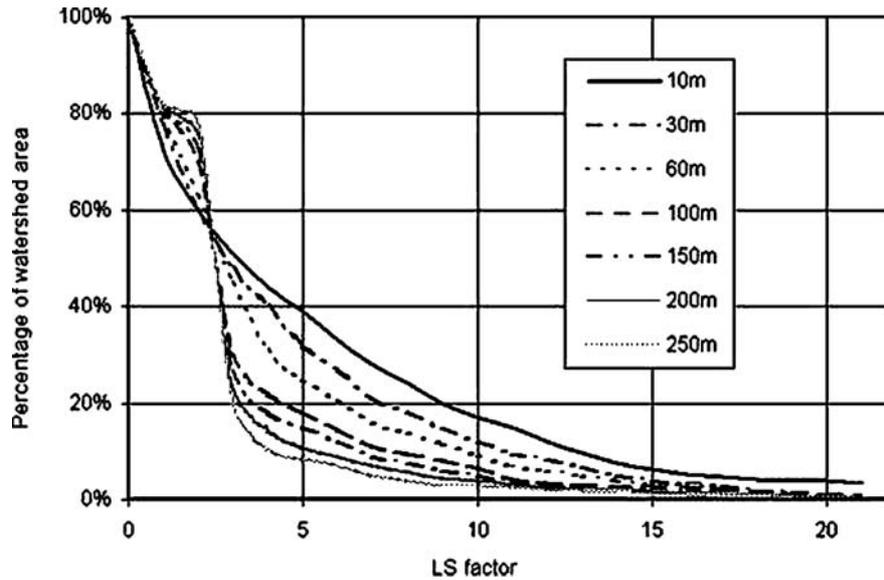
Figure 5. Cumulative frequency distribution of the *LS* factor at different DEM resolutions.
