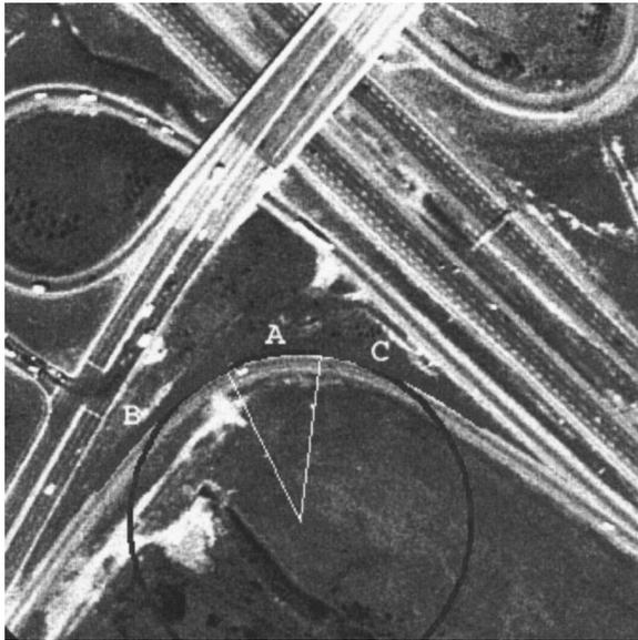
**Fig. 5.** Application 1: Extracting a spiralled horizontal curve (directional ramp)
