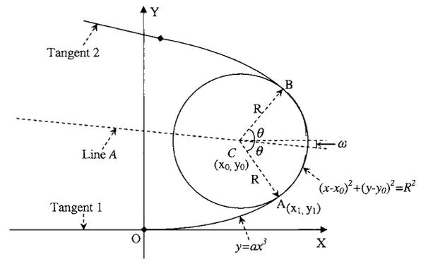
Fig. 2. Symmetrical horizontal curve with spiral approximated by cubic polynomial
