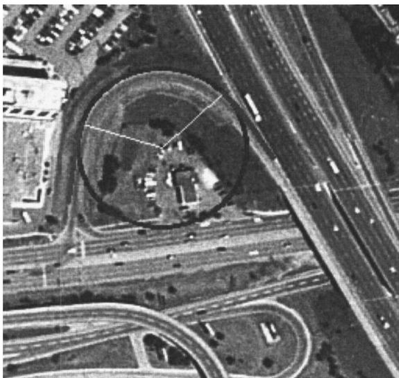
**Fig. 6.** Application 2: Extracting a spiralled horizontal curve (loop ramp)
