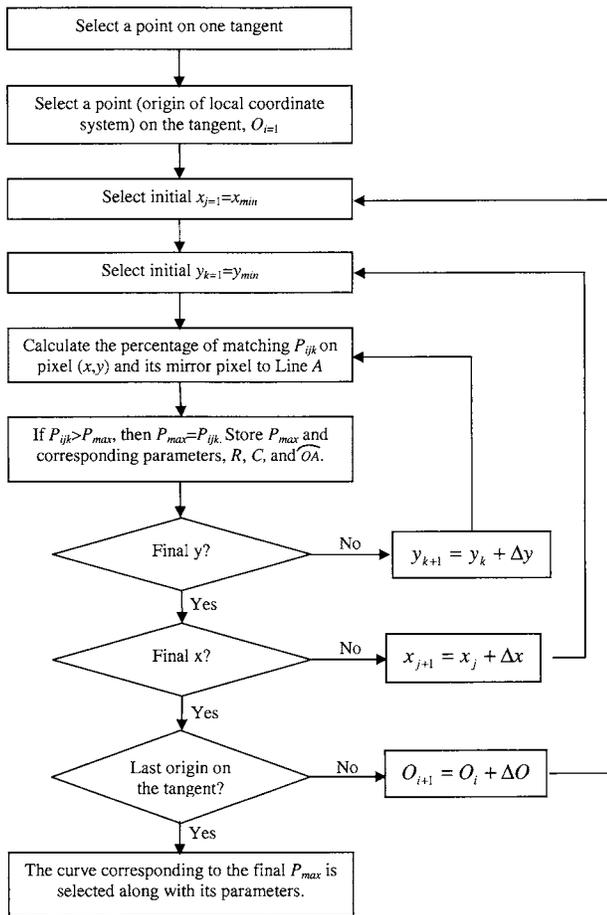
Fig. 3. Flow diagram for approximate extraction of spiralled horizontal curve
