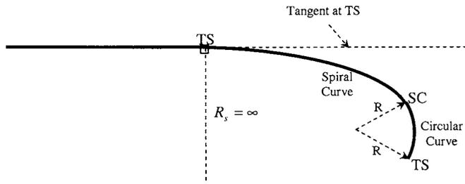
Fig. 1. Characteristics of spiral curve
