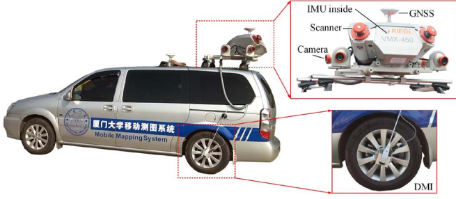
Fig. 7. Illustration of RIEGL VMX-450 MLS system and its components.
