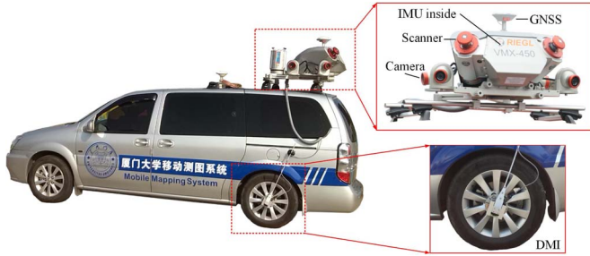
Fig. 9. Illustration of the RIEGL VMX-450 MLS system and its components.
