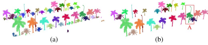
Fig. 4. (a) Clustering result of off-ground points, and (b) cluster filtering result using prior knowledge.
