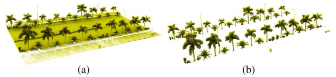
Fig. 3. (a) Raw point cloud, and (b) off-ground points after ground removal.
