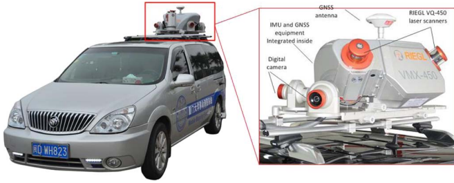
Fig. 1. RIEGL VMX-450 system with an inset picture of the laser scanners, cameras, and the navigation system mounted on the roof rack.
