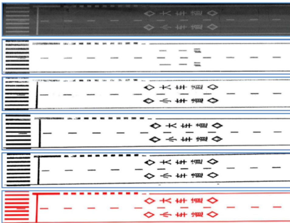
Fig. 16. Extracted road markings from Sample 05. From top to bottom: road surface point, Chen’s result, Guan’s result, Yu’s result, result of proposed method, and manually labeled benchmark (adapted from [24]).
