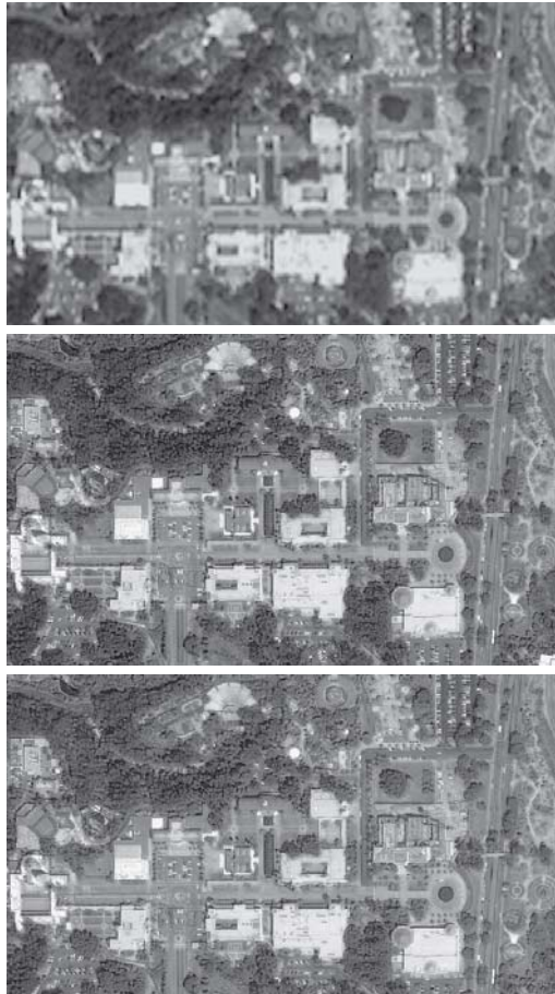
Fig. 4 Colour enhancement of Ikonos natural colour image. Top: original Ikonos colour image; Middle: pan-sharpened Ikonos colour image; Bottom: pan-sharpened and colour enhanced Ikonos image.
