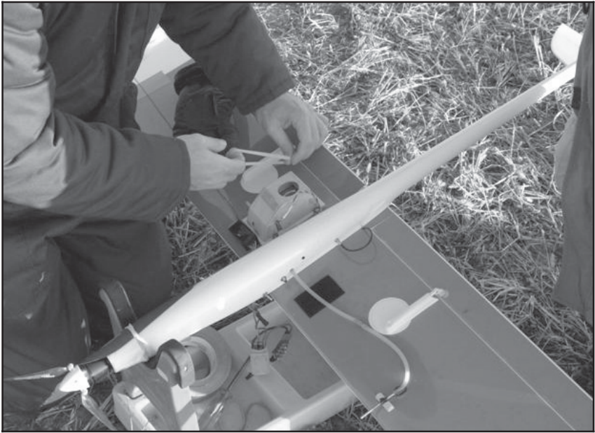
Fig. 3 Detail of the camera mounting system
