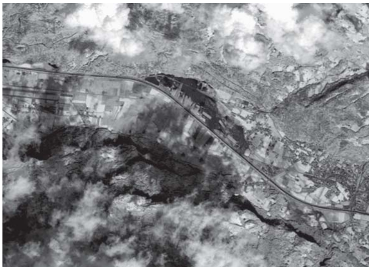
Fig. 2 A section of the SPOT5 near-infrared band showing the spectral similarity of flooded areas and shadows
