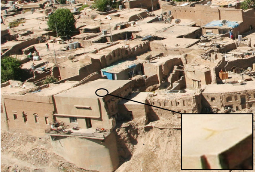
Fig. 3.6 Details of aerial photos from a helicopter flight (2006) with provisory created control point for photogrammetrical mapping (Photographed by K. Pavelka in 2006)
