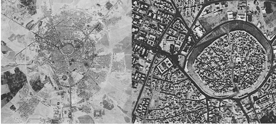
Fig. 3.4 (a) (left) – Corona satellite system (KH-4B); 16.8.1968; (b) (right) – details of the citadel – geometrical resolution approximately 3 m; very good quality (Source: USGS)
