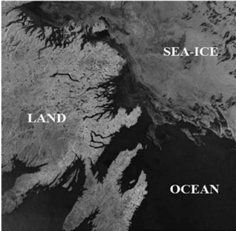
Fig. 6.5 RADARSAT-2 image (7,291 × 7,296 pixels) covering the sea area nearby the Island of Newfoundland in Canada, ScanSAR Wide beam mode, HH polarization, taken at 22:29:36 on March 16, 2009
