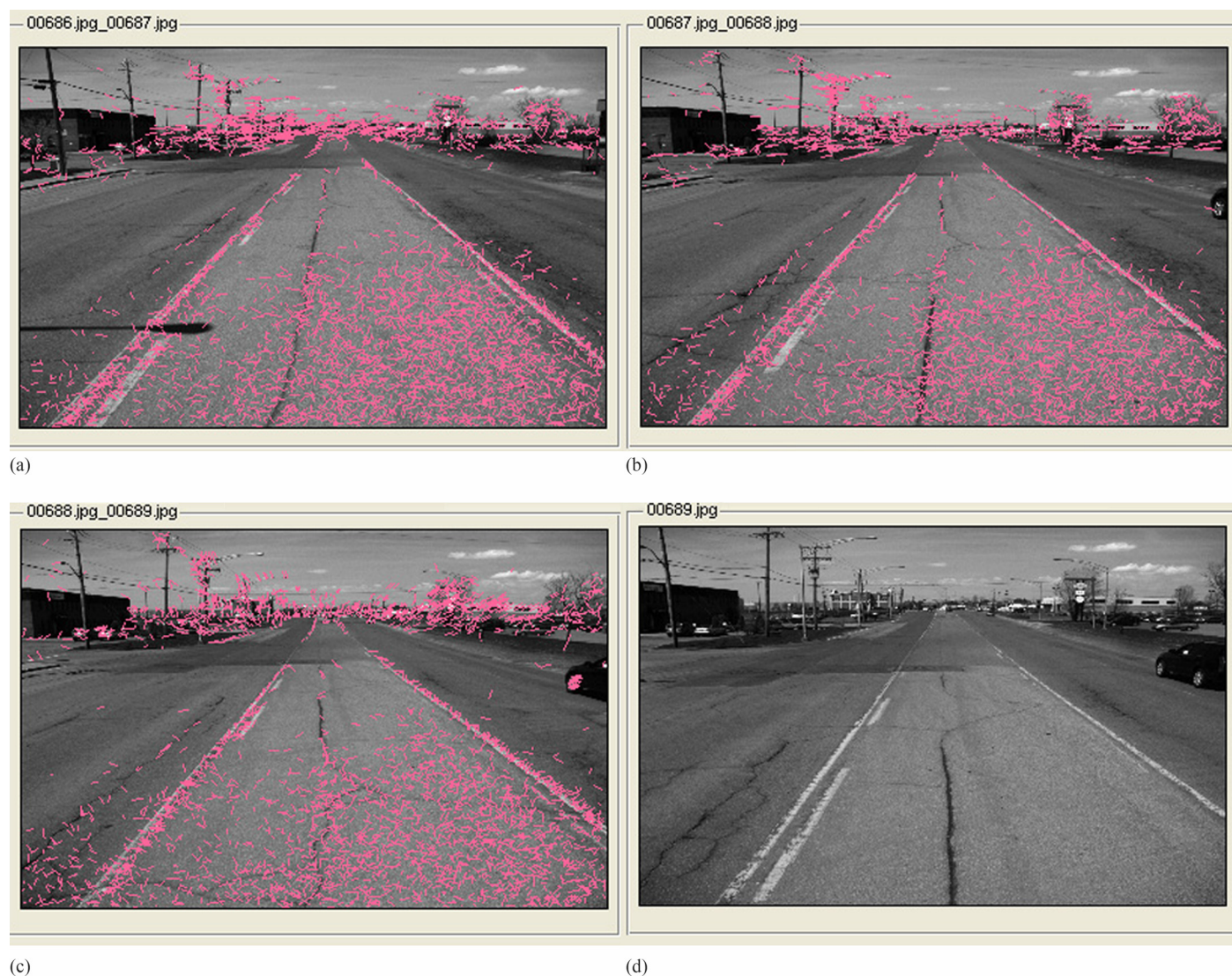
Fig. 4. Subplots (a) through (c) show homologous pairs of points, and (d) shows the original image: (a) between Frames 686 and 687 shown in Frame 686; (b) between Frames 687 and 688 shown in Frame 687; (c) between Frames 687 and 688 shown in Frame 688; (d) original image in Frame 689
